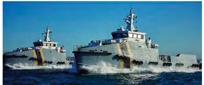
35m Sentinel crew & patrol vessels by Nautic: 28 knots, ballistic protected, fly-by-wire. 30 days of mission time between resupplies.
